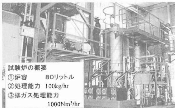
Fig. 4 Plasma-Induction Melting Test Facility
