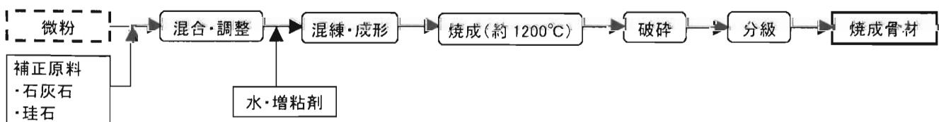
Fig. 20 Manufacturing process of sintered aggregates
