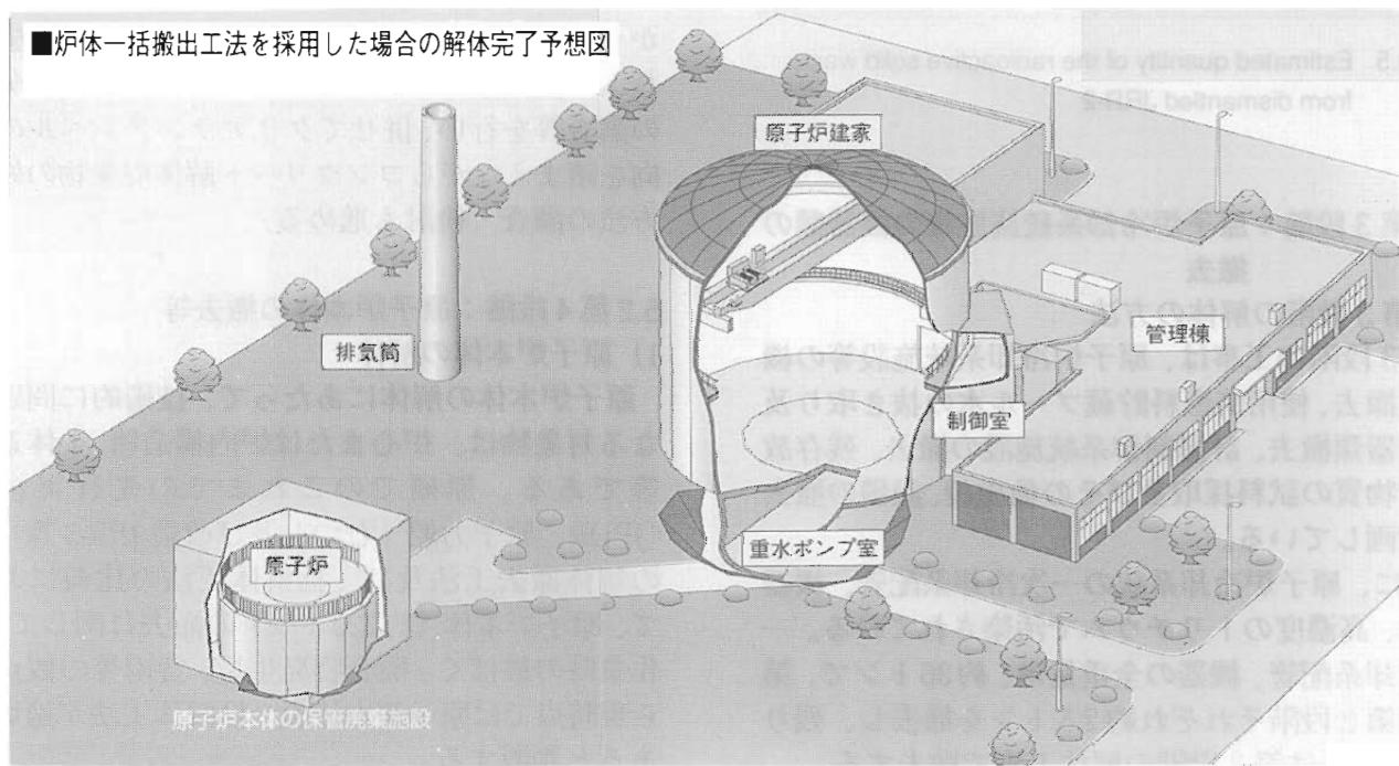
Fig. 7 Image of the dismantled reactor building, adopted “one-piece reactor removal method”
