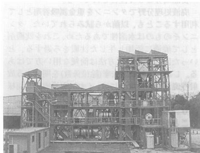
Fig. 18 Mobile type plant with 3t/h feed rate (verification plant of NEDO)
