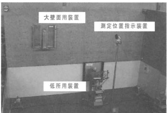
Fig.14 Image of Wall Measurement using Double Layer Array Type  $\beta$  /  $\gamma$  Detector and Support Equipments
