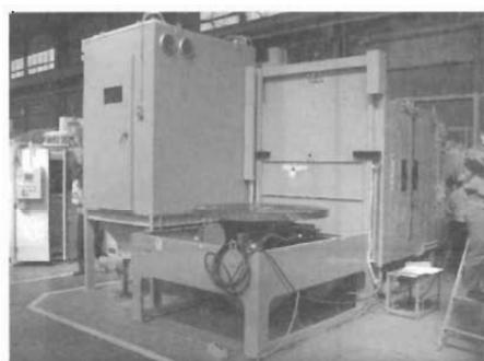
Fig.17 Zirconia Blast Decontamination Equipment
