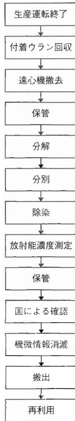
Fig.10 Treatment of Used Centrifuge
