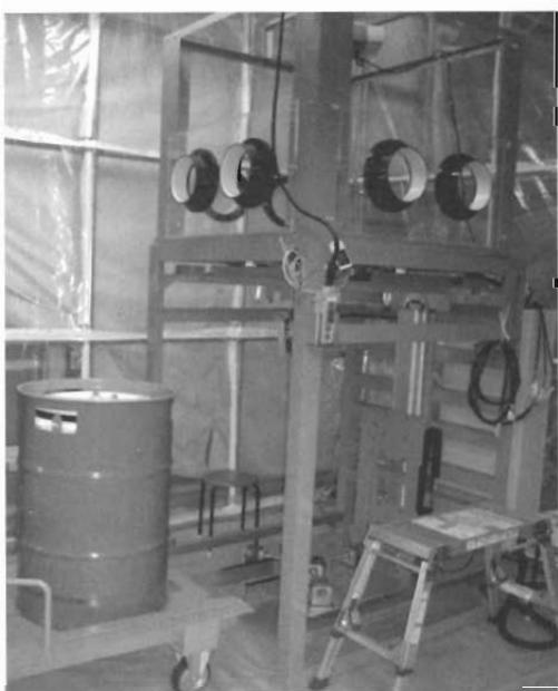
Fig.10 Direct in Drum System for Radioactive Waste
