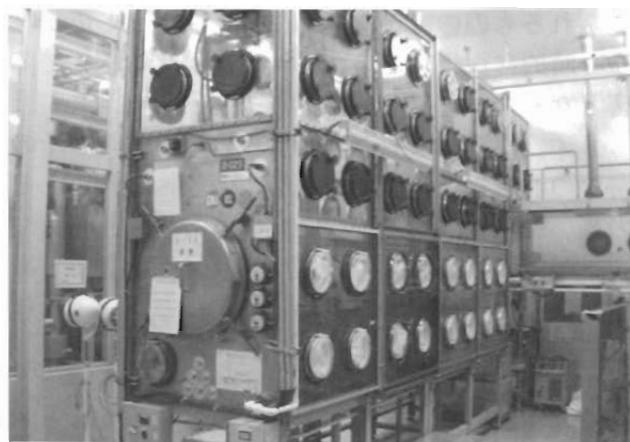
Fig.2 Glovebox for MOX Fuel Fabrication
