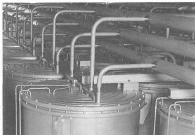
Fig.6 Metal Cylinder Centrifuge
