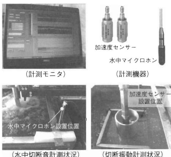
Fig.6 Measuring Sounds and Vibrations Generated during the Cutting
