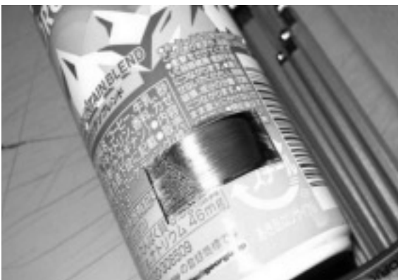
Fig.8 Expanded View after the Laser Peeling, as Focused just on the Surface of the Can. As the Laser Spot Area in the Left side of the peeled is larger than the Right one, the removed layer thickness of the left side is smaller than the thickness of the right side.
