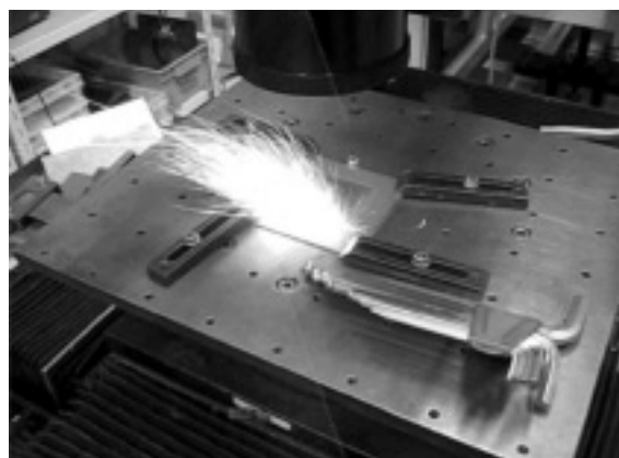
Fig.6 Laser Peeling Tests for a Flat and Shiny Stainless Steel Plate.
