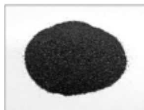
Fig.4 Blast material (High hardness stainless steel grain)
