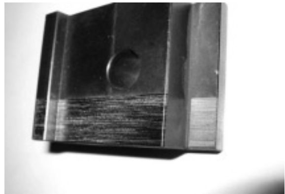
Fig.9 Automatic Surface Peeling of the 3 Stepped Carbon-Steel Block.
